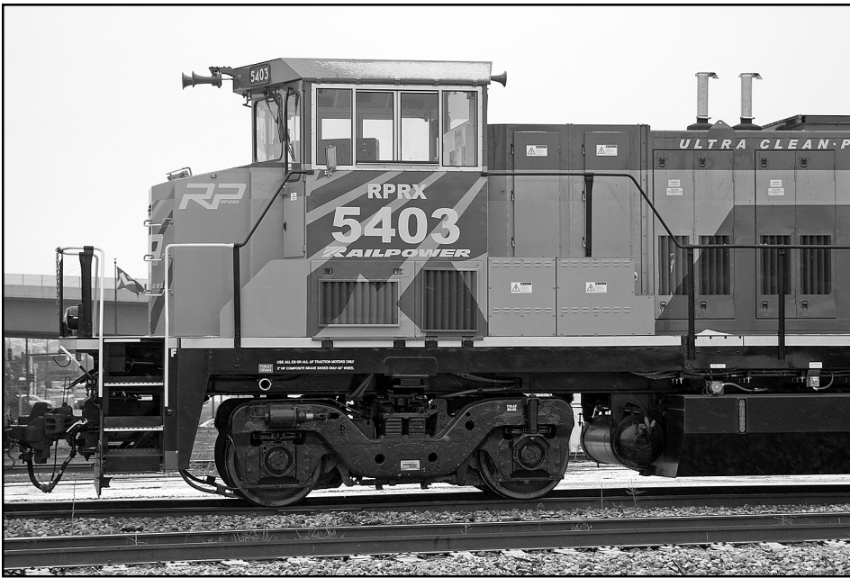
Freshly outshopped RailPower model GG20B 5304 has high visibility cab. Unit was stopped at Prospect Junction as the Casper, WY, to Amarillo, TX, train worked out a distributed power link problem with the rear DPU. – Photo © 2007 by Chip.
